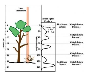
Figure 7. Full waveform system.
