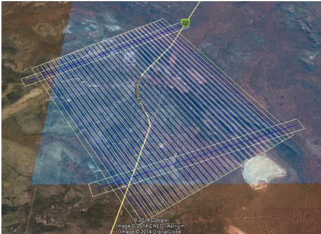
Figure 4. Flight path with 70% front to back overlap and 60% sidelap.
