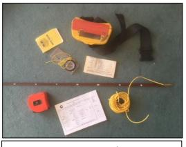
Figure 6: Monitoring tools. (Notebook, Hip Chain, Compass, Pocket map, Measuring pole, tape measure and nest data sheet).
