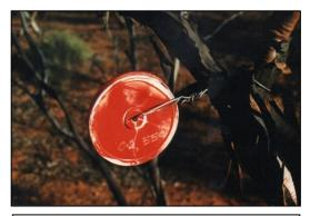
Figure 5: Red reflector on its wire mount with melted written coordinates.
