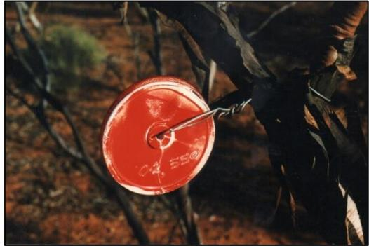
**Figure 5: Red reflector on its wire mount with melted written coordinates.**
